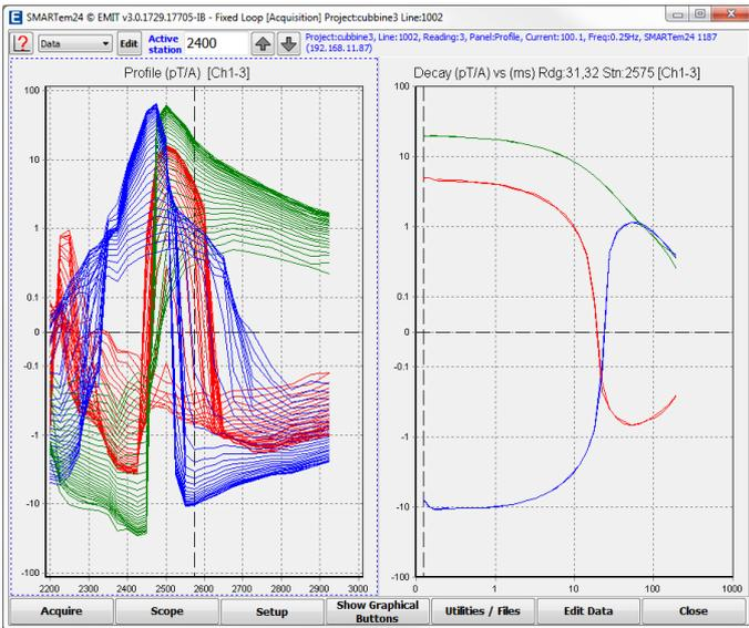
**SMARTem24 software showing Profile and Decay panels from a SMART Fluxgate survey**
