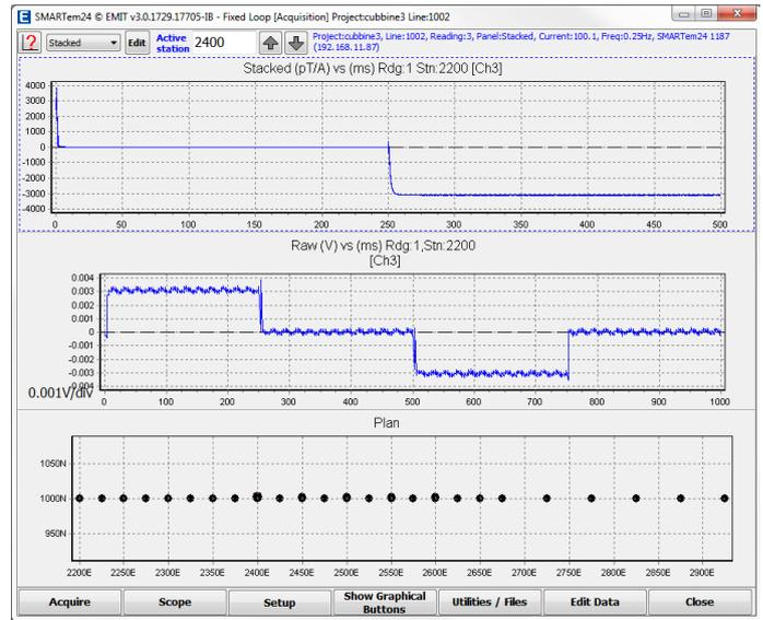
**SMARTem24 software showing Stacked, Raw and Plan panels from a SMART Fluxgate survey**
